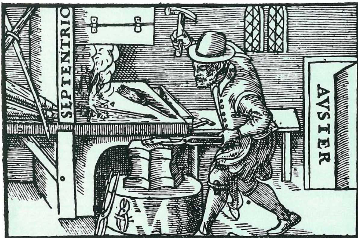
Fig. 1. In the 1600's, William Gilbert discovered that a magnet could be made by heating an iron bar, then letting it cool in the direction of the earth's field.
